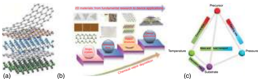
Figure 7.1 (a) Van der Waals hybrid structures. Source: Geim et al. [32]/Macmillan Publishers Limited. (b) Overview of the 2D materials using CVD growth, from single crystal to 2D material-based hybrid structures and their applications. (c) Schematic showing how various parameters affect the kinetics in the growth of 2D materials. Source: Reprinted with permission from Cai et al. [33]/American Chemical Society.
