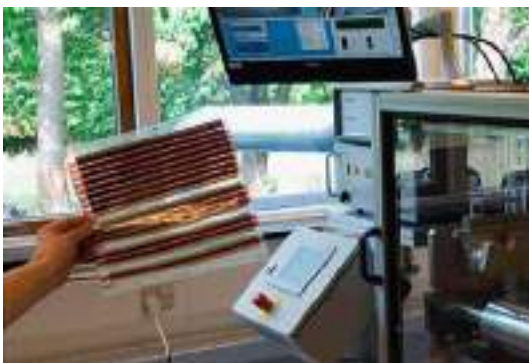
Figure 6.15 One of the completed modules in front of the R2R coater. Source: Krebs et al. [149], Elsevier.
