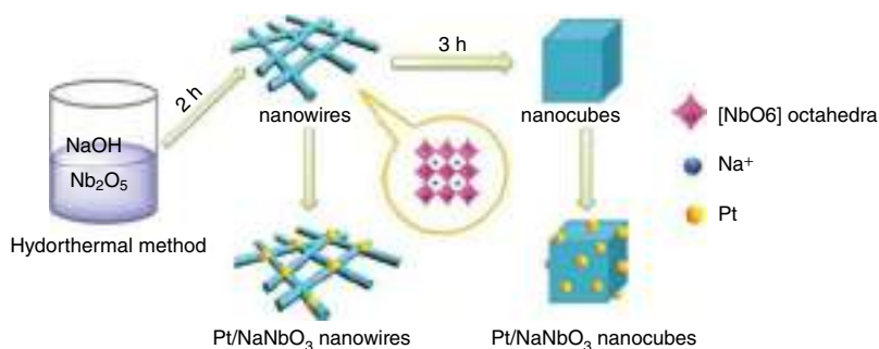
Figure 6.9 The catalysts' formation paths, which include a network of corner-shared octahedral units of [NbO 6 ]. Source: Liu et al. [132]/with permission of Elsevier.
