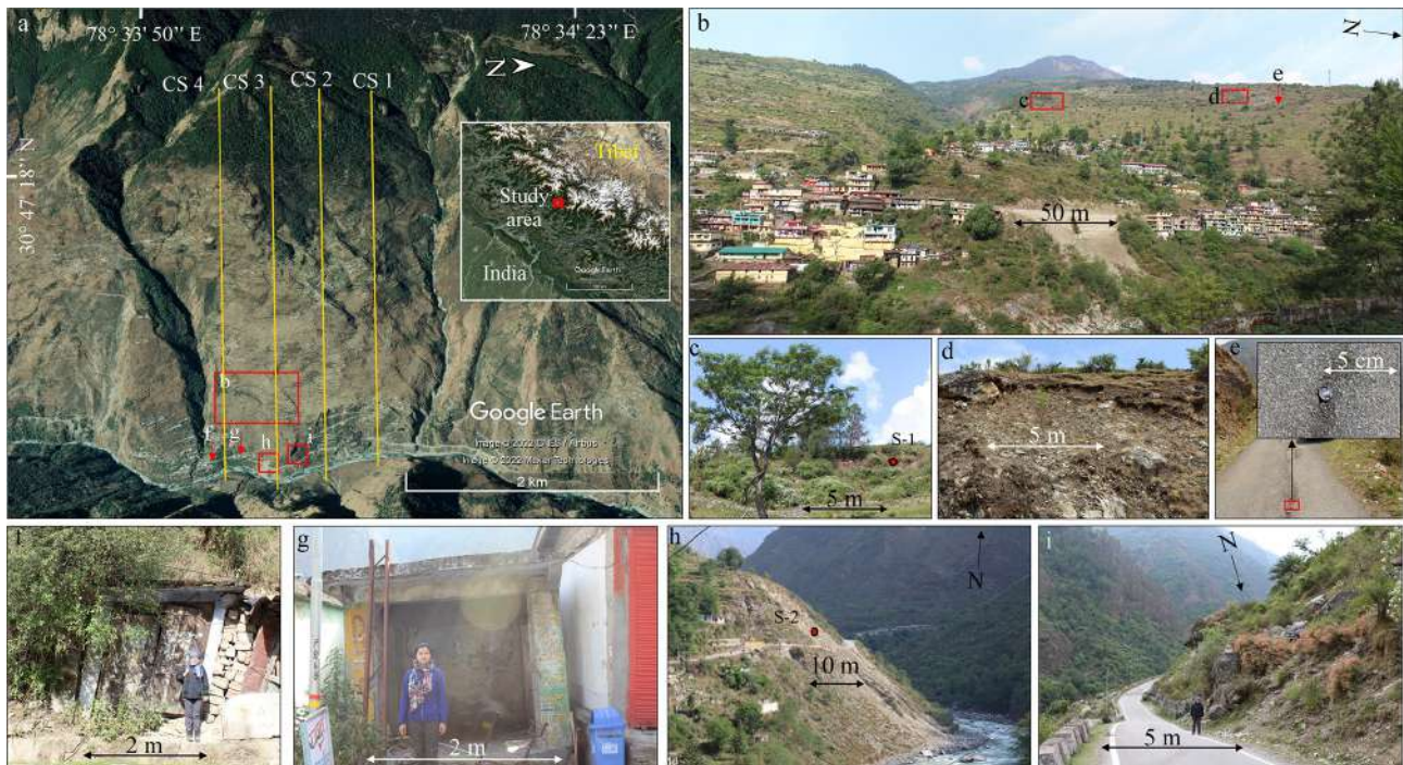
Figure 2. Field observation of Bhatwari. © Google Earth for panel (a). (a) Location of Bhatwari with the inset highlighting its position in the NW Himalaya. CS 1 to CS 4 mark the position of 2D slope sections used for the slope stability evaluation. (b–d) Exposed scarp. S-1 refers to the soil sampling site, (e) cracks and displacement of the road, (f–g) tilting houses and shops, (h) active slope failure at the slope toe, and (i) big gneissic boulder implying a paleo-landslide site.
