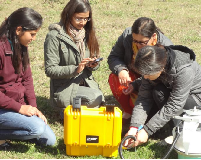
SENR Research scholars working with LICOR soil respirometer
